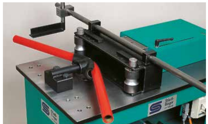
132 Cintrage de tubes "Gaz" Gaspijp buigen
