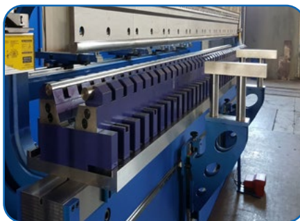
Adjustable V-die system, CNC or manually adjusted (optional)
