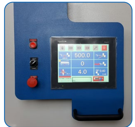
Color Touch Screen 10.4", movable along machine's length (optional)
