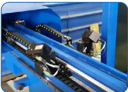
i-measure: Laser measurement of the bending angle and real time correction (optional)
