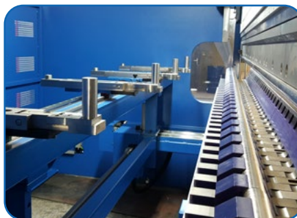
Special made finger stop for thick material (optional)
