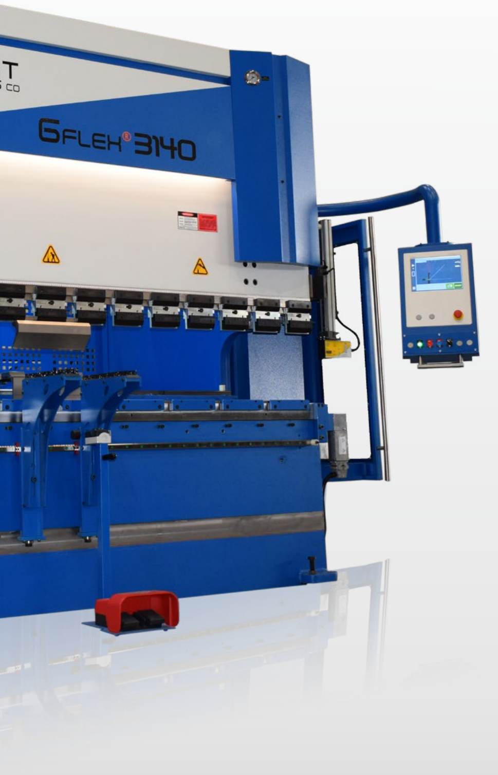
2D graphic Controller, 12" Touch Screen, CybTouch12, including Touch Profile function and automatic bend sequence calculation.
