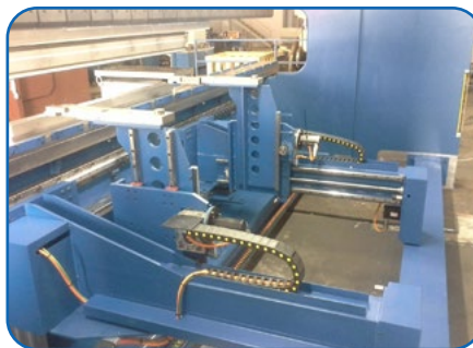
6-axis back gauge, X1-X2-R1-R2-Z1-Z2 (optional)
