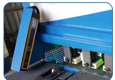
Finger protection with light guards (optional)
