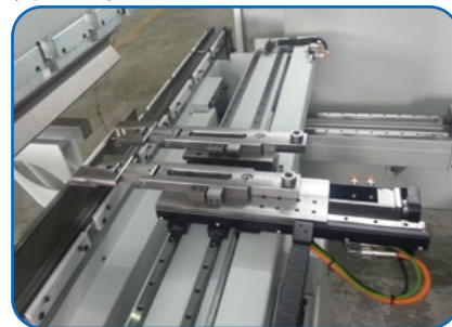
5-axis back gauge, X-X'-R-Z1-Z2 (optional)
