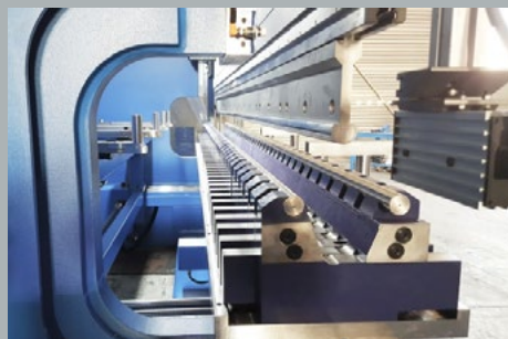
Special, heavy-duty, adjustable die, V=25 - 400mm.
