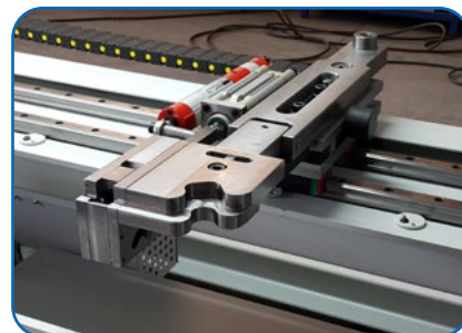
Automatic Thickness Measurement (ATM) and Bending Program Correction (optional)
