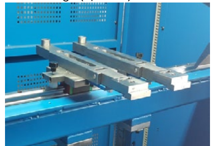
Hydraulic Wila Clamping, with vertical tool change (optional)
